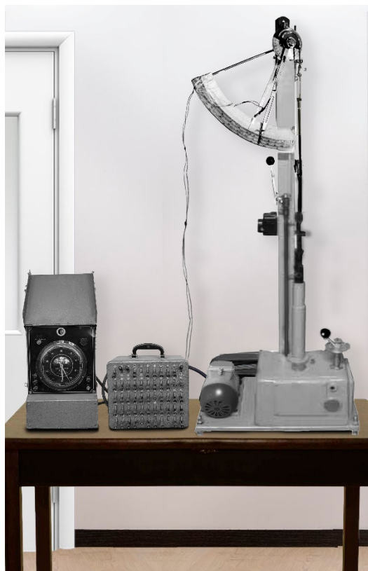
Fig. 1. The general view of the device for testing the samples made from the cane stem
