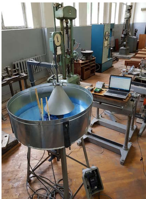
Fig. 2. The general view of the experimental plant for the plants vibration cutting in the water medium.
